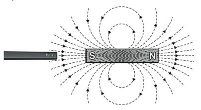
The x-direction measurement is positive when the wand points toward the South pole of a magnet.
