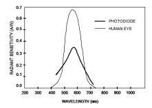
**UV-BLUE Sensor**: The UV-BLUE sensor uses the difference in readings between two photodiodes. One photodiode has a wide response including the UVA region, and the other is only sensitive to visible light. The difference creates a response primarily in the UVA region, but it does extend slightly into the blue end of the visible light spectrum. This sensor will provide a non-zero response to some deep-blue (but visible) light sources, such as fluorescent light bulbs.
