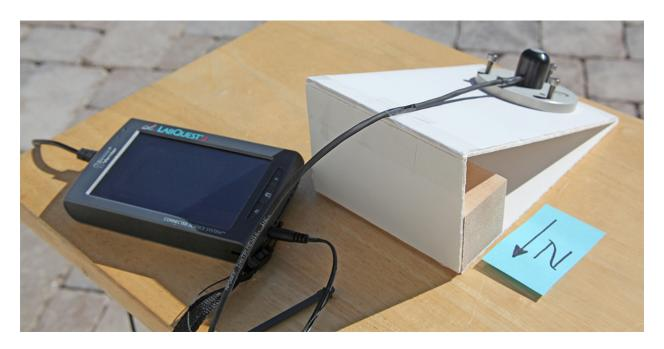
Logger *Pro* was then used to compute the total electromagnetic energy delivered by the sun to the panels for each of the seven hours under investigation. The chart below shows this in watts-seconds per square meter for each of the seven hours (9:00 a.m. through 4:00 p.m.), obtained as the area under the Irradiance *vs.* Time chart from the Pyranometer.
