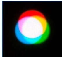
For subtractive color mixing, a diverging cone of light is produced and the screen adjusted until it is evenly illuminated with white. Typical positions have the lens 5 cm from the light source and the screen 30 cm from the lens.
