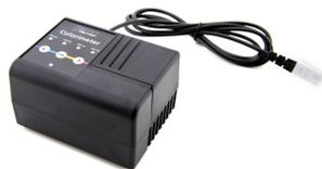
The Vernier Colorimeter is used to determine the concentration of a solution by analyzing its color intensity. The cuvette slot is designed to accommodate most cuvettes with a 10 millimeter path length. The Colorimeter measures the amount of light transmitted through a sample at a user-selectable wavelength. You may choose from four wavelengths: 430 nm, 470 nm, 565 nm, and 635 nm. Features such as automatic sensor identification and one-step calibration make this sensor easy to use.
