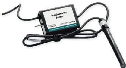
The Conductivity Probe can be used to measure either solution conductivity or total ion concentration of aqueous samples being investigated in the field or in the laboratory. Conductivity is one of the most common environmental tests of aquatic samples. Even though it does not tell you specific ions that are present, it quickly determines the total concentration of ions in a sample.
