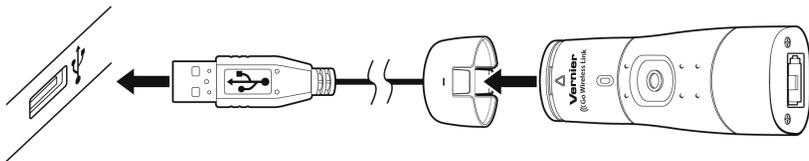
You can also charge up to eight Go Wireless Link interfaces using our Go Wireless Charging Station, sold separately (order code: GW-CRG). An LED on each Go Wireless Link indicates charging status. A blue light indicates it is still charging. When the light goes off, it is finished charging.
