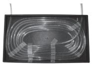
Cover the tubing in the box with the clear plastic lid. You can tape one edge onto the box to make a hinge, or tape all the edges for a tight seal.
