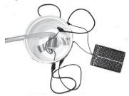
Next, pour water into the container. Use room temperature water so that you can measure a temperature change as the system operates. The water pump should be fully submersed, but keep the wires sticking up out of the water so you can connect the solar panel to the pump in Step 3.
