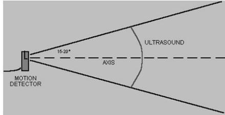
Note that the Motion Detector will report the distance to the closest object that produces a sufficiently strong echo. The Motion Detector can pick up objects such as chairs and tables in the cone of ultrasound.
