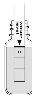
small white reference contacts near the tip of the electrode should be immersed. Make sure no air bubbles are trapped below the ISE.
