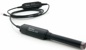
The Vernier Optical DO Probe can be used to measure the concentration of dissolved oxygen in water samples tested in the field or in the laboratory. The Vernier Optical DO Probe is a luminescence-based optical oxygen sensor. This technology reduces the need to calibrate the sensor and no stirring is required since it does not consume oxygen.
