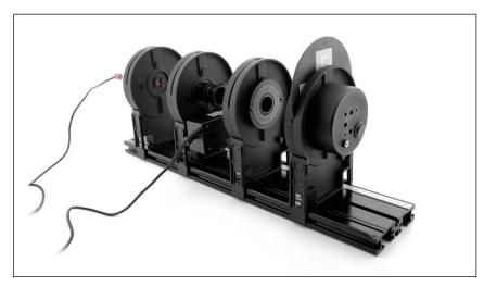
Modified assembly with the Adjustable Analyzer for Rotary Motion Sensor and a Light Sensor
