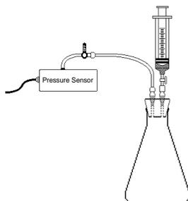
Erlenmeyer flask and close the valve. Vapor pressure data can easily be collected using any of our interfaces and data collection programs. Gently swirl the flask. Once the system equilibrates, the flask can be placed in water baths of varying temperature to investigate the relationship between vapor pressure
