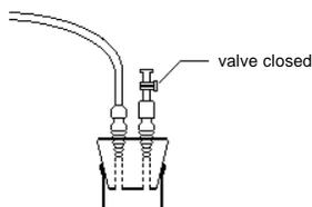
shown here. For example, when doing a pressure-temperature experiment, the tubing apparatus can be connected to the rubber stopper which is in turn inserted into the neck of a 125-mL Erlenmeyer flask:
