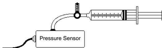
The white, threaded adapter end of the long piece of plastic tubing can also be connected to one of the valve stems with a full turn. The other end can be connected to the shorter stem on the two-way stopper included with your Pressure Sensor, as
