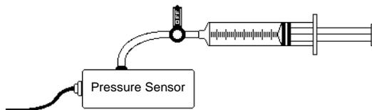
The pressure inside the syringe is now equal to atmospheric pressure at the volume you selected. You are now set to collect pressure-volume data. Take data as you change the volume. The syringe is marked in volume units (cc or mL). You can both increase and decrease the volume. This experiment is detailed in our *Chemistry with*
