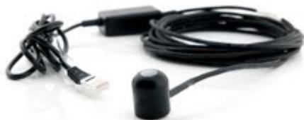
The Vernier Pyranometer measures the power of electromagnetic radiation in watts per square meter. It is sensitive to the near infrared, visible, and UV ranges, where nearly all of the solar energy is concentrated. It is great for experiments with solar cells and calculating their efficiency. The sensor is weatherproof and has a dome-shaped top to allow it to work with a wide range of sun angles. The Pyranometer has a 6 m cable.
