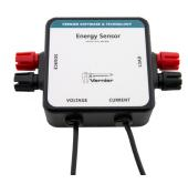
These terminals will accept standard banana plugs, alligator clips, or bare wires and provide a solid electrical connection.
