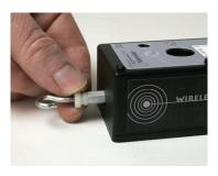
The hook connected to the force sensor
