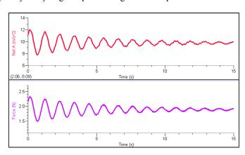
Force and acceleration graphs made with a WDSS suspended by a rubber band (Damped harmonic motion)
