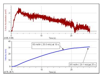
Acceleration of an automatic transmission car
