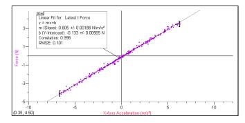
Force vs. acceleration with linear fit
