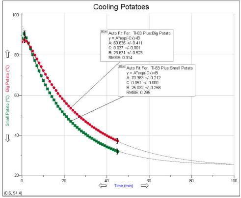
These data were recorded using a LabPro interface and a TI-83 Plus Silver Edition calculator. The data were transferred over to Logger *Pro* 3 for analysis.
