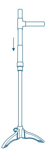
3. Fit the Tee assembly into the base assembly.
