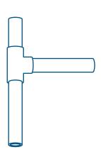
3. Attach the 3" PVC and the two smaller 6" PVC pieces to the Tee fitting as shown.
