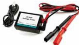
The 30-Volt Voltage Probe is used to measure electrical potentials in the range of  $-30$  to  $+30$  Volts. This sensor uses an internal voltage divider connected to the  $\pm 10$  volt input of the interface. Use this sensor in experiments that involve voltages larger than 10 Volts, such as when working with large solar panels.
