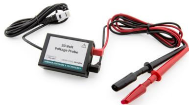
The 30-Volt Voltage Probe is used to measure electrical potentials in the range of  $-30$  to  $+30$  Volts. This sensor uses an internal voltage divider connected to the  $\pm 10$  volt input of the interface. Use this sensor in experiments that involve voltages larger than 10 Volts, such as when working with large solar panels.
