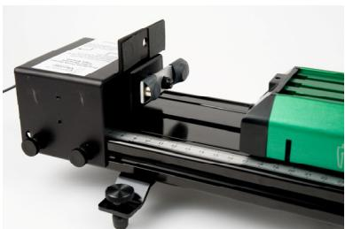
2) Sensor on Cart – Another way to collect the data is to attach a single magnet bumper to the up turned tab of the Track Bracket. (The single magnet can be attached using the small nut that holds the dual-magnet bumper to the Track Bracket.) Attach another single magnet bumper to the DFS and attach the DFS to the cart. Give the cart a gentle push toward the Track Bracket.
