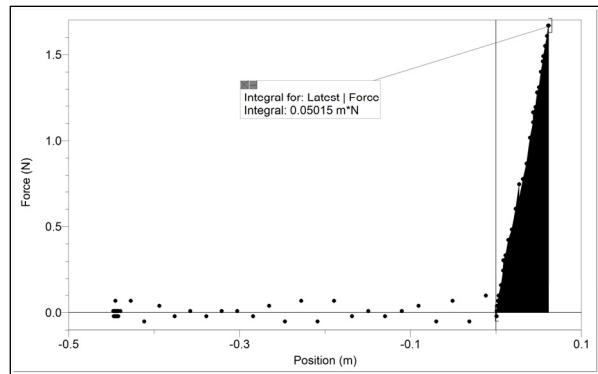
If you don't have *Logger Pro* software or if you don't want to use the integral function of the software, you can simply calculate the area of the triangle created by that set of data.
