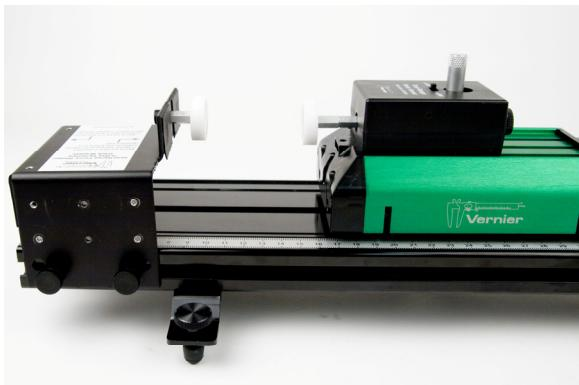
3) Collision with a contact force – Perform the same experiment described above, but instead of the magnets put a loop bumper on the track bracket or the cart.
