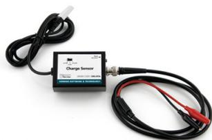
The Charge Sensor is used as an electronic electroscopes. Unlike a traditional electroscopes, the Charge Sensor can make quantitative measurements. Numerical measurements improve many electrostatics experiments, such as charging by induction, charging by friction and charging by contact. The sensor can also be used to measure charge polarity.
