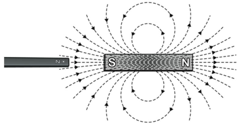
*The x-direction measurement is positive when the wand points toward the South pole of a magnet.*
