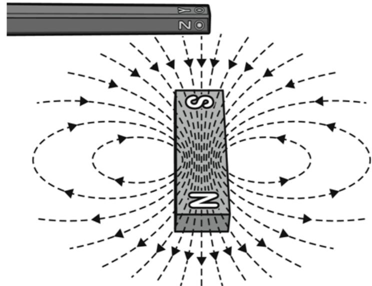
*In this orientation, the z-direction measurement will be positive.*
