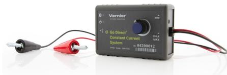
The Go Direct Constant Current System is a DC power source with a built-in current probe designed for use in electrochemistry experiments. The user can set the current by tuning the dial. The system is capable of delivering up to 0.6 A. The following is a partial list of activities and experiments that can be performed using this sensor.
