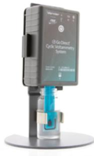
Go Direct Cyclic Voltammetry System is a potentiostat that students can use to easily control and apply potential to a chemical system and measure the response as electrical current. It has three modes of data collection: cyclic voltammetry, bulk electrolysis, and open-circuit potentiometry. It includes a stand, scintillation vials, and disposable screen-printed electrodes. Free Vernier Instrumental Analysis<sup>®</sup> software and free experiments are available for download.
