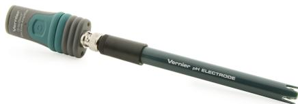
Go Direct pH can be used for any lab or demonstration that can be done with a traditional pH meter, including acid-base titrations, monitoring pH in an aquarium, and investigating the water quality of streams and lakes.
