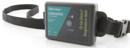
Go Direct Respiration Belt uses a force sensor and an adjustable nylon strap to measure respiration effort and rate. An LED indicator provides feedback so belt tension can be optimized for best results. Respiration rate is reported within the software, which makes comparison studies between subjects or experiments easy to do. The sensor can also be used to measure steps and step rate. The following are some activities and experiments that can be performed using the Go Direct Respiration Belt:
