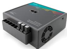
Go Direct Fluorescence/UV-VIS Spectrophotometer is a small, lightweight ultraviolet and visible light spectrofluorometer. It is a combined fluorometer with a UV-VIS absorbance spectrometer. Exchangeable LEDs ensure you get the exact excitation wavelength needed.
