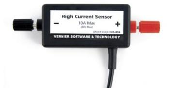
The High Current Sensor is used to measure current in the range of  $-10$  to  $+10$  A. The sensor uses a Hall Effect chip, so that it does not add a resistive element to your circuit. A replaceable fuse protects the equipment and circuit. Use the sensor in experiments that involve currents larger than 1 A, such as solar panels, hand generators, etc.
