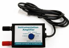
Our Instrumentation Amplifier is used to condition signals to be compatible with Vernier interface products. The amplifier provides the necessary gain and offset to allow you to connect a wide variety of measurement equipment to your interface and electronically collect, store, and analyze the data.
