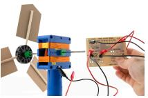
AC power source to the AC side of the Bridge Rectifier; connect wires from the DC side to the Visual Voltmeter to read the voltage output of your power source. **Note:** Using the Bridge Rectifier introduces about 0.5 V drop in power output. For instance, a 2 V AC input will become a 1.5 V DC output.
