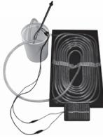
This Solar Thermal Exploration Kit is modeled after a domestic solar water-heating system. How you design the solar heating system will dramatically affect how quickly the water will heat and the maximum temperature the water will reach. The kit allows you to explore variables such as box color, light intensity, tube design, rate of water pumping, and amount of time it takes to heat the water.
