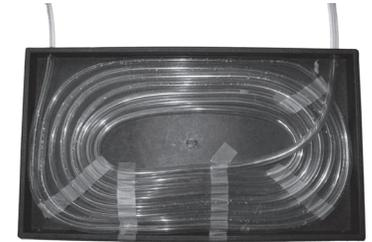
Cover the tubing in the box with the clear plastic lid. You can tape one edge onto the box to make a hinge, or tape all the edges for a tight seal.
