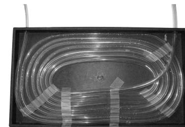
Cover the tubing in the box with the clear plastic lid. You can tape one edge onto the box to make a hinge, or tape all the edges for a tight seal.
