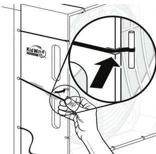
Plug all the fans into a power strip. Fans can be individually adjusted at the motors, although we recommend using the high setting. The average wind speed is approximately 3.6 m/s at a distance of 30 cm from the opening.
