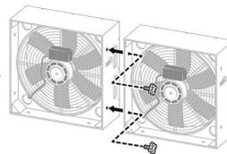
Assembled correctly, the fan speed adjustments are located in the tunnel. The rubber feet of the upper units fit into the holes on top of the lower units, and the handle holes face outside toward the back. Bungee tie slots are around the sides and top of the assembled fan wall. There are threaded holes on the inside sides and bottoms of each wind power unit. The holes line up and are meant to lock the fan walls together using the connecting screws.
