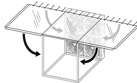
After you have secured the hook-and-pile fasteners along the edges, stretch the bungee cord connections into the fan wall notches. Start with the center top and work your way across and down to the bottom corners.
