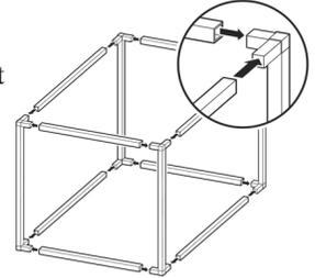
Don't worry if the frame seems a little wiggly or loose. Make sure all the tubes are pushed into the hubs. When the vinyl covering is put on, it will compress the frame and tighten it up.
