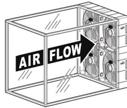
The wind speed of the wind tunnel is very sensitive to exterior obstructions and airflows. Ideally, it should be set up in an interior space and away from any outside fans or ducts. An 8' x 10' clear area in front and in back is desirable.
