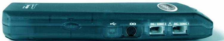
Serial Port and Digital Channels (USB Port is behind the sliding door)
