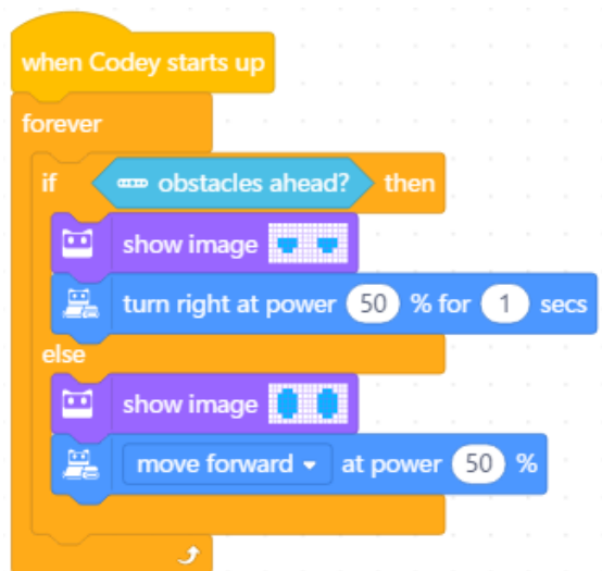
FIGURE 4 Simple obstacle avoidance program in mBlock 5 software; in mBlock app, the "when green flag clicked" hat block replaces "when Codey starts up."
