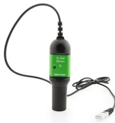
The O<sub>2</sub> Gas Sensor can be used to monitor gaseous oxygen levels in a variety of biology and chemistry experiments. The sensor is intended for measuring gaseous, not aqueous, O<sub>2</sub> concentrations.
