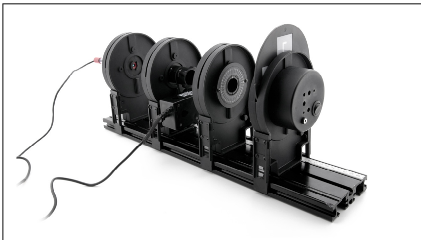
Modified assembly with the Adjustable Analyzer for Rotary Motion Sensor and a Light Sensor
