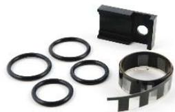
The Photogate Bar Tape Kit contains a flexible plastic tape called Bar Tape and a guide that allows the tape to be used with a Vernier Photogate. The tape is 3 m long, and it has alternating opaque and transparent bars with spacing of 1.524 cm. The tape can be attached to objects and pulled through the photogate. This allows you to perform experiments much like what you would do with a “ticker tape timer”.
