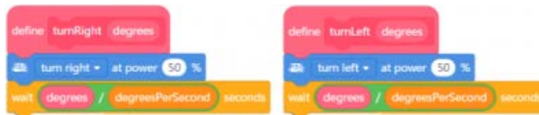
FIGURE 6 "turnRight" and "turnLeft" blocks turn mBot right and left, respectively, in much the same way the "moveDistance" subroutine drives mBot forward.
