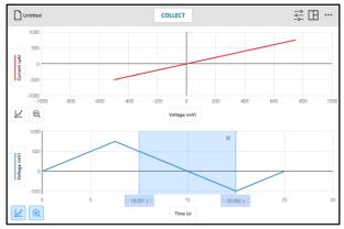
The absolute value of the slope of the linear fit should match the CV sweep rate.
