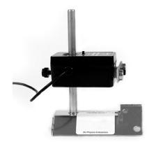
Use the U-shaped adapter and nylon thumbscrew/nut to secure the magnetic bumper to the air track glider. For PASCO gliders, use the bracket with two banana plugs. For Central Scientific & Daedalon gliders, use the long bracket and four 10-24 screws. Alignment of the magnetic bumpers is critical. The magnets on the DFS should be 1-2 mm higher than the glider magnets for best results.
