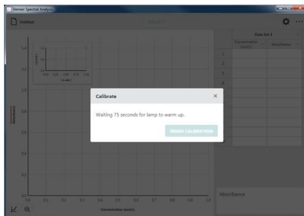
3. When the lamp warm up is complete, place a blank cuvette in the holder with the clear sides aligned with the arrow on the spectrometer. Click or tap **FINISH CALIBRATION** to complete the calibration.
