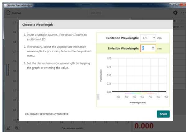
3. Select the Excitation Wavelength you are using for your experiment. The wavelength options shown depend on the spectrometer you are using.
