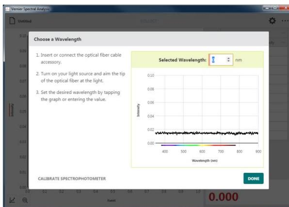
3. If needed, click or tap CALIBRATE SPECTROPHOTOMETER and follow the onscreen instructions to calibrate the spectrometer.
