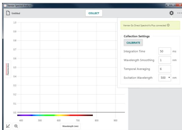
3. Adjust the Excitation Wavelength to select the wavelength you want to use. The wavelength options shown depend on the spectrometer you are using.
