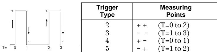
The crossover point between the two computations is about 600 Hz. Because there can be a one-count uncertainty during the 0.25-second period, the accuracy around 600 Hz is approximately  $\pm 4$  Hz (about 0.7%). The resolution of the timer measuring the time between edges is 6.4 microseconds; therefore, the percentage accuracy improves for frequencies above and below 600 Hz.
