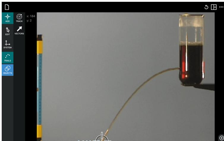
*Figure 1 Collecting data for the water stream along the bottom edge of the video*
