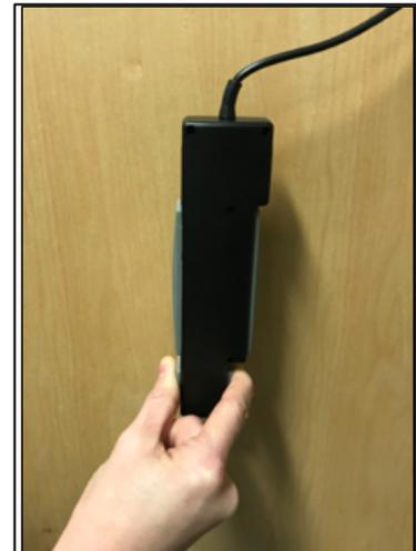
Figure 15. “Pinching” the Dynamometer.
