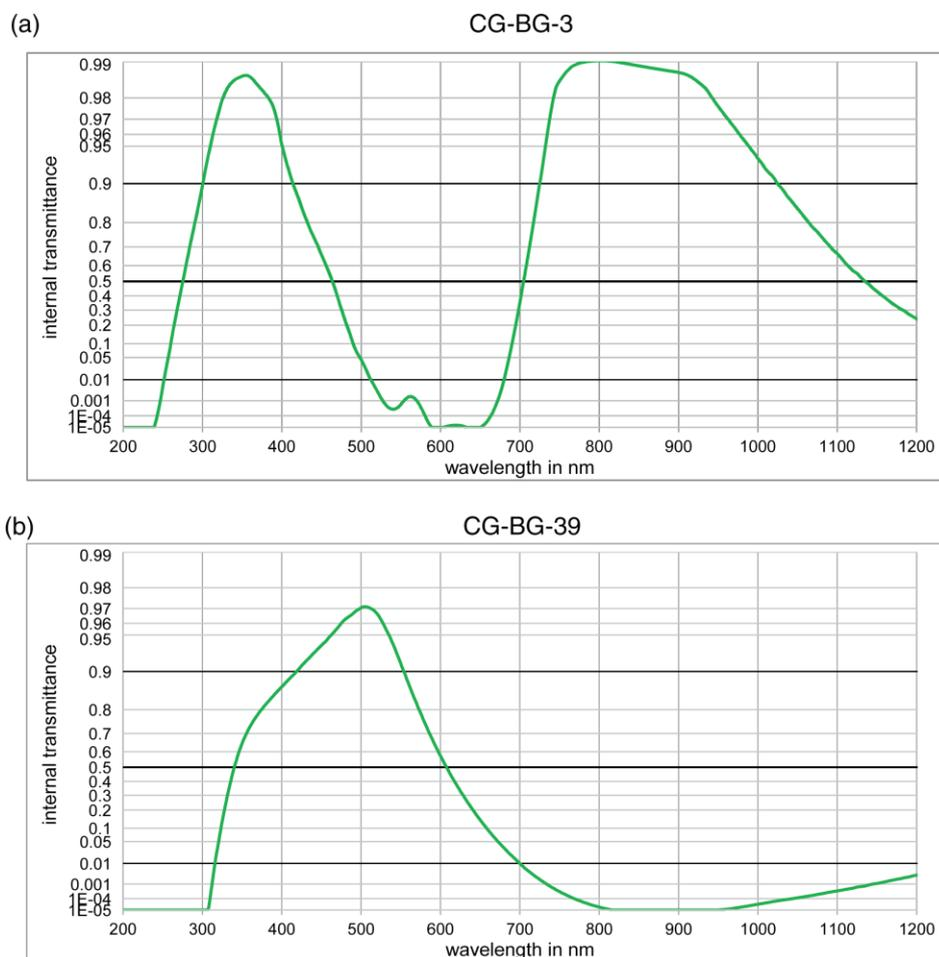
Figure 5: Transmission spectrum of (a) CG-BG-3 filter and (b) CG-BG-39 excitation colored glass filters
