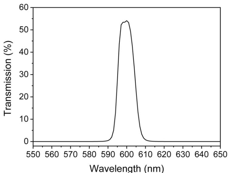
Figure 6: Transmission spectrum of 600 nm detection dielectric interference filter.
