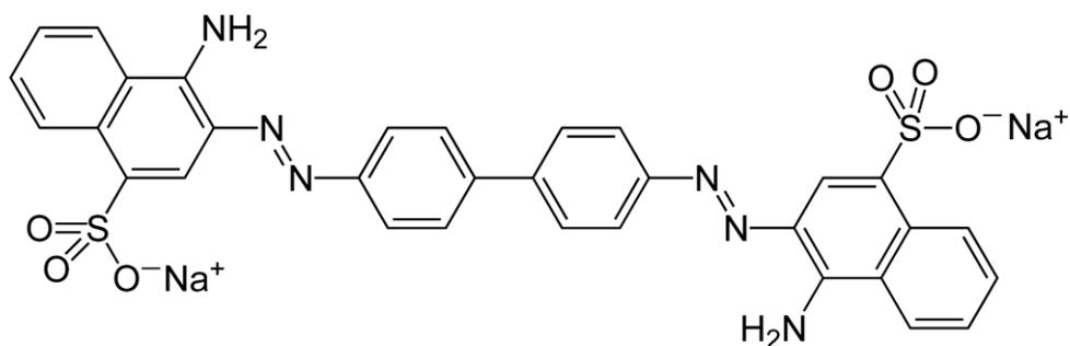
Figure 8: Skeletal structure of Congo Red, molecular weight = 696.67
