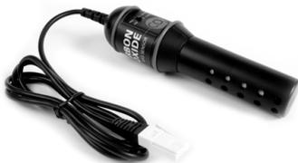
The Vernier CO<sub>2</sub> Gas Sensor measures gaseous carbon dioxide levels by monitoring the amount of infrared radiation absorbed by carbon dioxide molecules.
